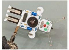
The circuit is powered by a 9V battery. The battery travels securely with the robot in its backpack, the battery holder.
