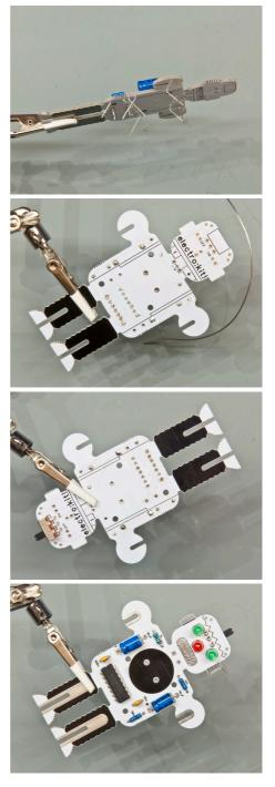
Repeat the same process as for the resistors and capacitors. Insert one component at a time; bend the leads, double check the orientation, and then solder both leads.
