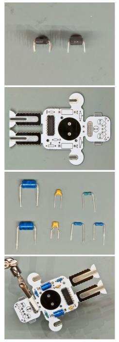
When all components are in the correct place and correct orientation, make one final inspection to make sure they are indeed in the correct place and correct orientation before soldering.
